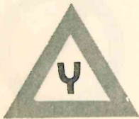
B. 3 DUAL CARRIAGEWAY AHEAD
