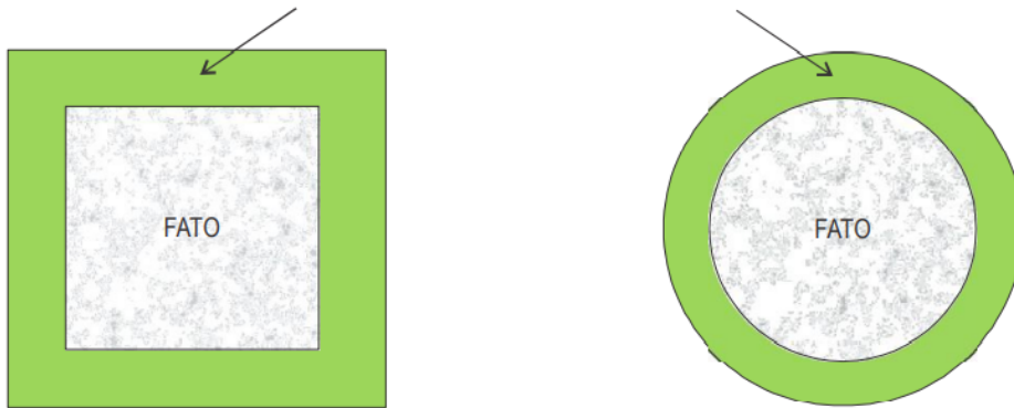
Figure 2-1. FATO and associated safety area
